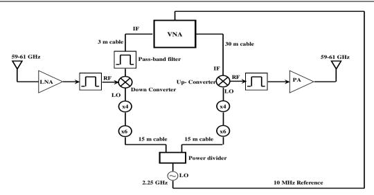
Fig.2 Measurement set-up
