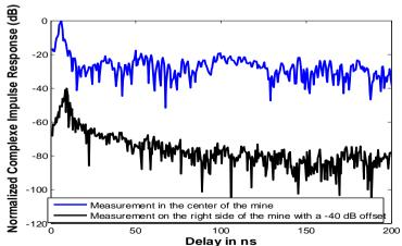
Fig 2 Normalized power delay profile at a distance of 1.6 meters for both scenarios.
